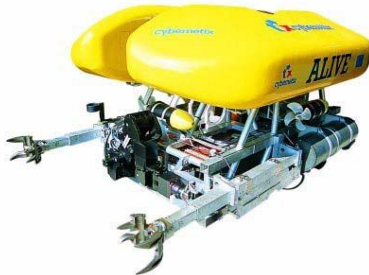
Figure 1-3 ALIVE autonomous Light Intervention vehicle by Cybernetix
