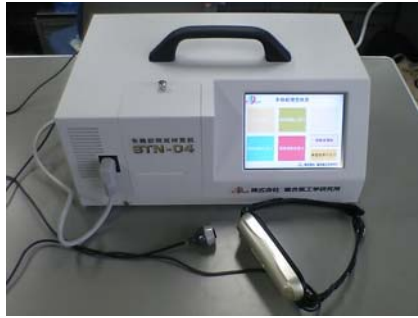
Figure 2-8 Multifunctional sight inspection apparatus (STN-04)
