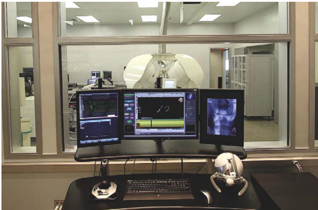
Figure1- 6 Catheter Guidance Control and Imaging' (CGCI) system
