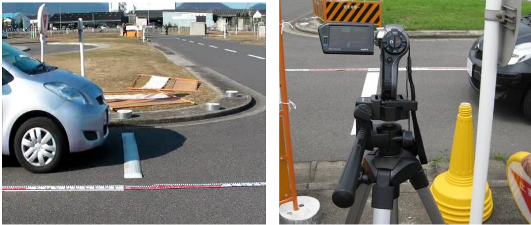
(a) Graduated ruler to measure stopping position (b) Video camera to record stopping behaviors
