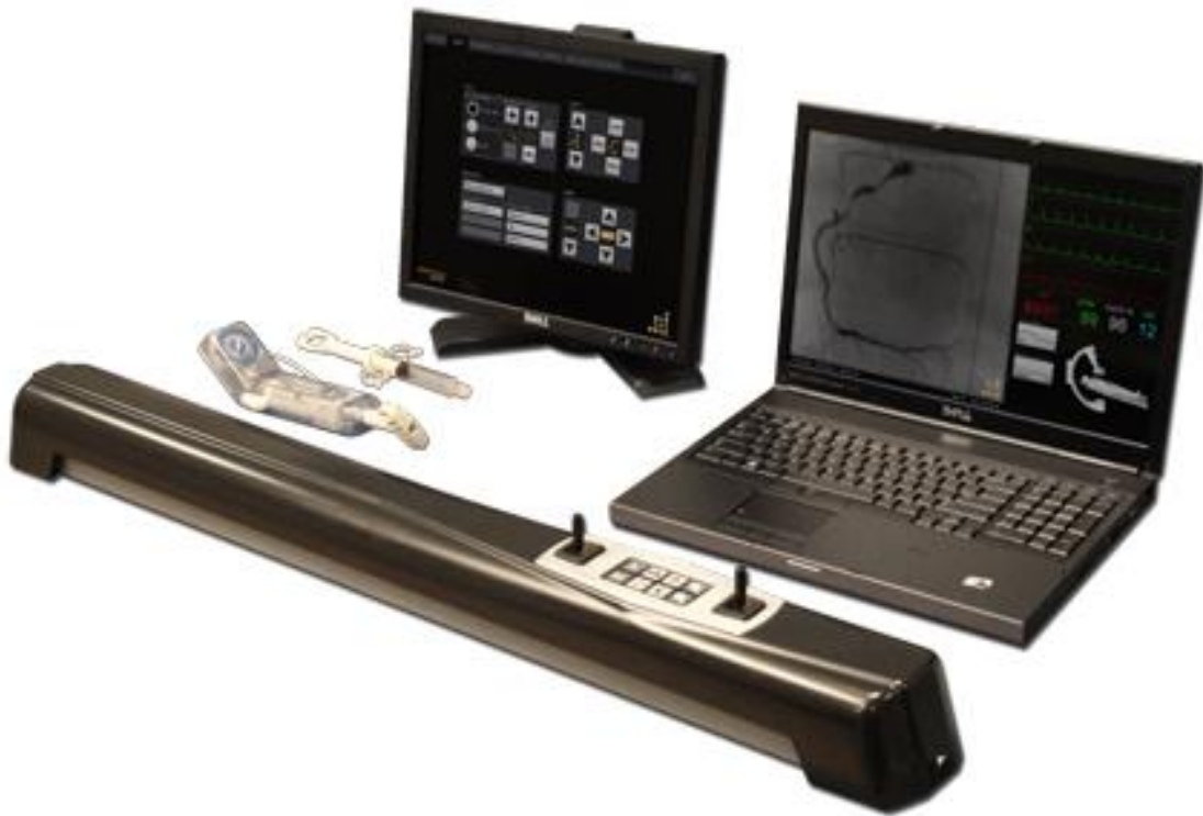
Figure1- 9 the Procedicus Vascular Interventional System Trainer [VIST, MenticeAB]
