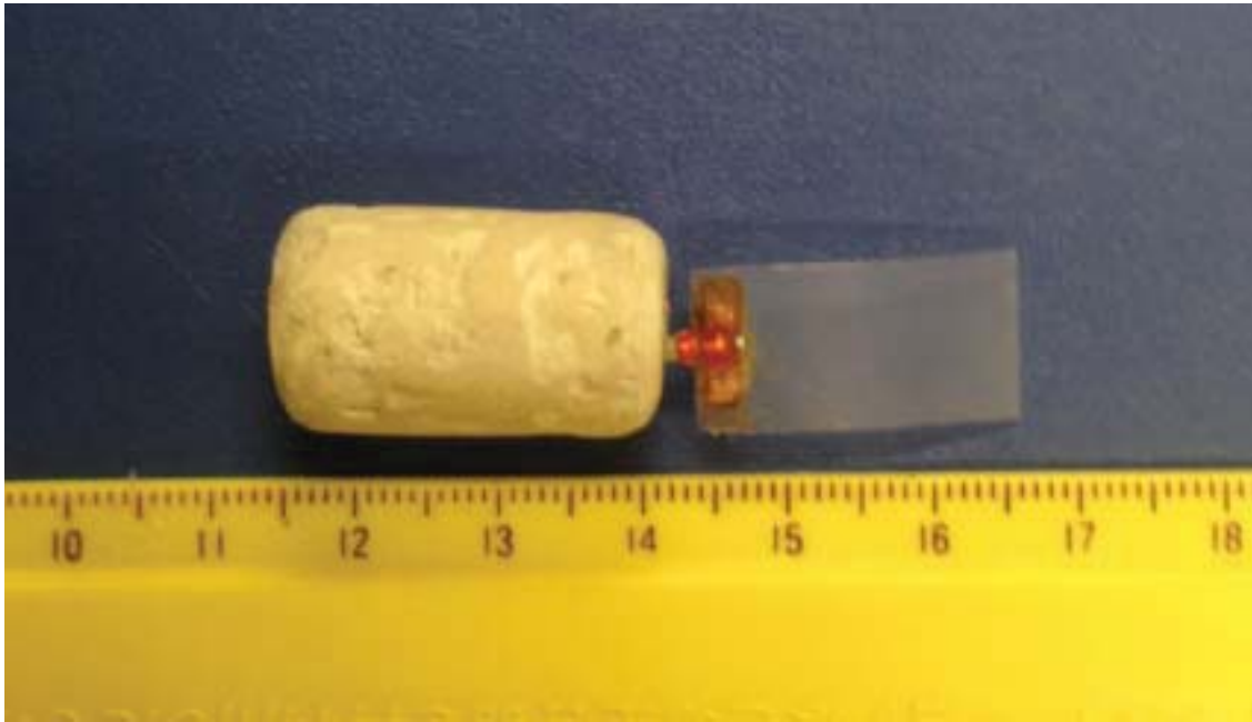
Figure 4.2 Prototype of the magnetic actuated hybrid microrobot
