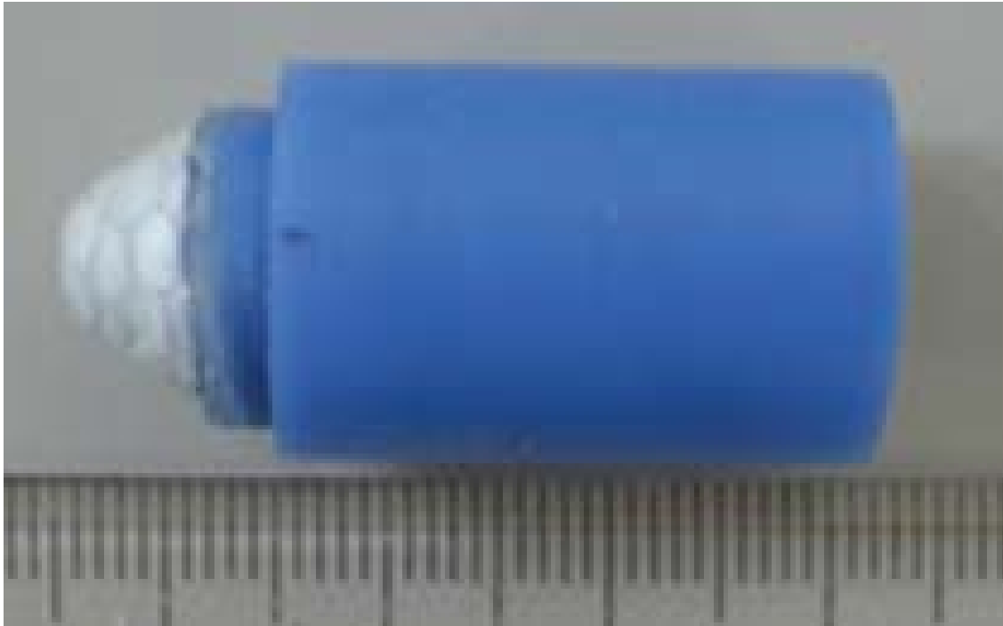
(a) Prototype of magnetic actuated microrobot with screw jet motion
