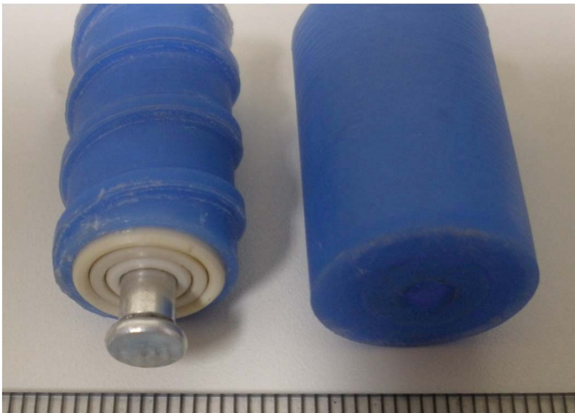
(b) A bare propeller and a non-rotating nozzle
