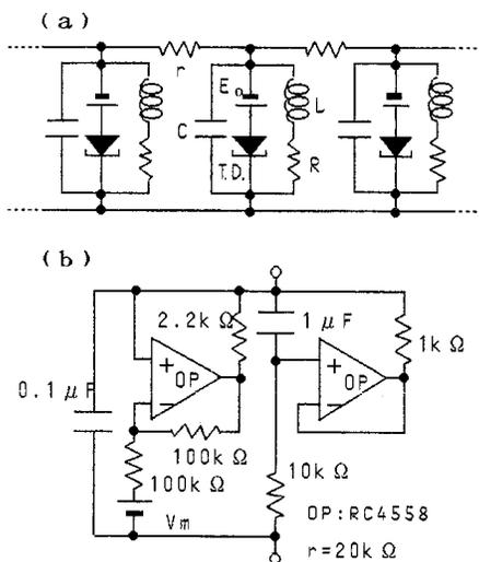
Fig. 4 Nagumo's active transmission line (a) and an analog circuit for one element with OP amps (b).
