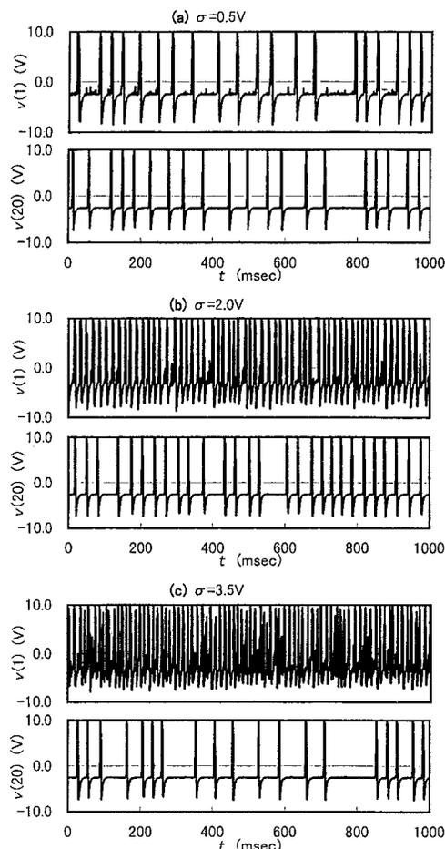
Fig. 5 Time series of the voltage in the noise-added (1st) element and 20th element with  $\sigma = 0.5$  V (a), 2.0 V (b) and 3.5 V (c) (Nagumo's active line).
