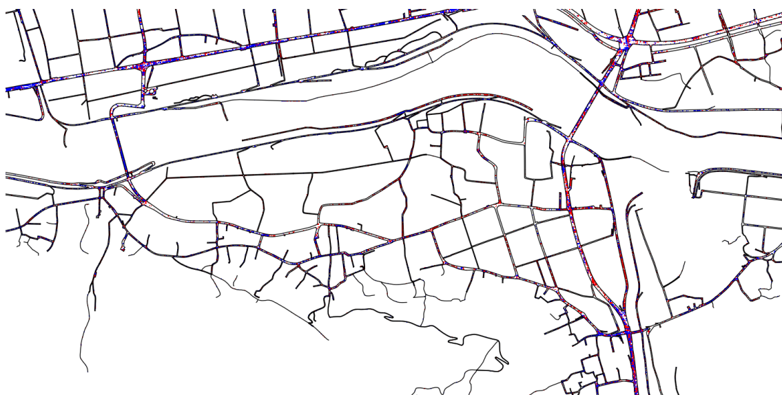
Fig.5.21 Extraction of damaged area on road (South side of Oda river)
